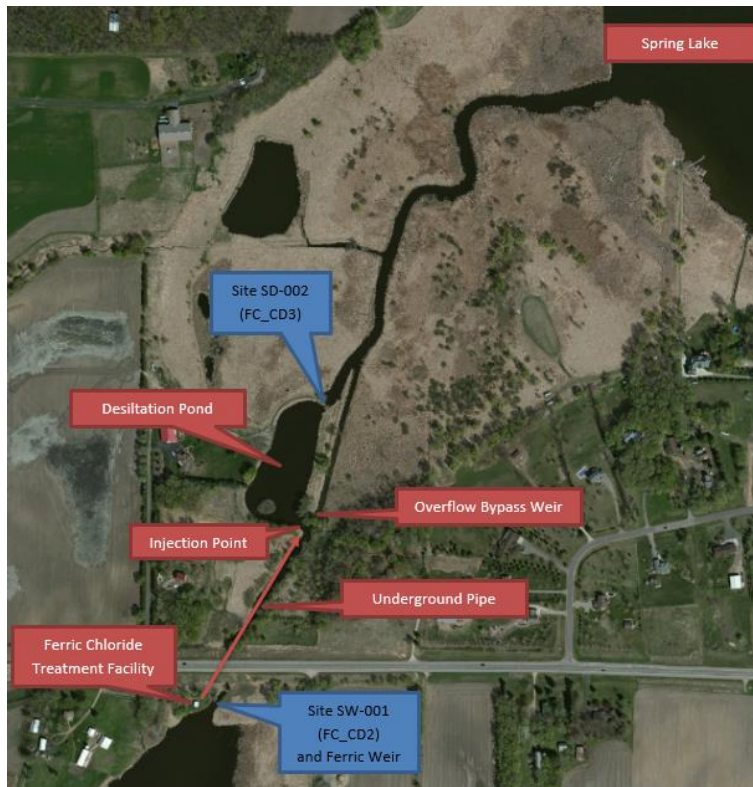
Figure 3. Aerial Map of Ferric Chloride Treatment System
